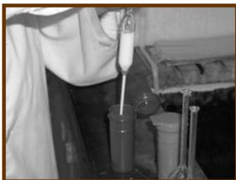
up to 8% fat. A cream test bottle will allow fat readings up to 50%. The smallest division of graduation of a milk test bottle represents .1 of one percent. A cream test bottle is graduated in .5 of one percent.
